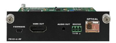
The PM-FR102-U-RF is a PureMedia™ Fiber Optic extender receiver designed for use with the RF4-U Rack-Mount Extension Center. The PM-FR101-U-RF offers powerful and reliable long-distance extension of Ultra HD/4K video, embedded and analog stereo audio, as well as control signals up to 32,808 ft. (10 km) over a single-mode fiber optic cable.
